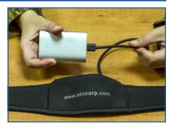
Press the power button on the "BATTERY" before placing the battery in the Neck/Shoulder strap battery compartment.
