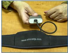
Once the battery has been activated, place it in the provided battery compartment in the center of the Neck/Shoulder strap and close the zipper.
