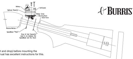
It is best if you adjust the stock fit (cast and drop) before mounting the SpeedBead. Your shotgun owners manual has excellent instructions for this.
