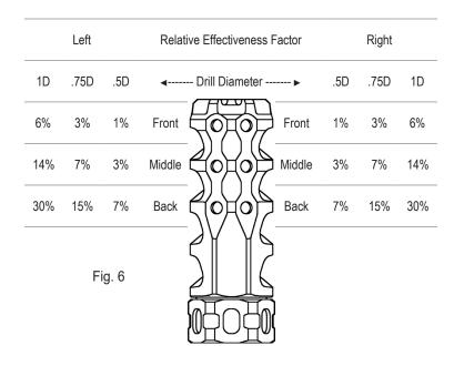
their opposing top holes. Note: Drilling the bottom holes may slightly increase ground disturbance when shooting prone. To minimize this always start with the forward hole locations first.
