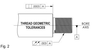
**IMPORTANT:** Fig. 2 outlines barrel thread geometric tolerances required for installation, most factory barrel threads should satisfy these requirements. For thread specifications and dimensions please visit: www.precisionarmament.com/manuals
