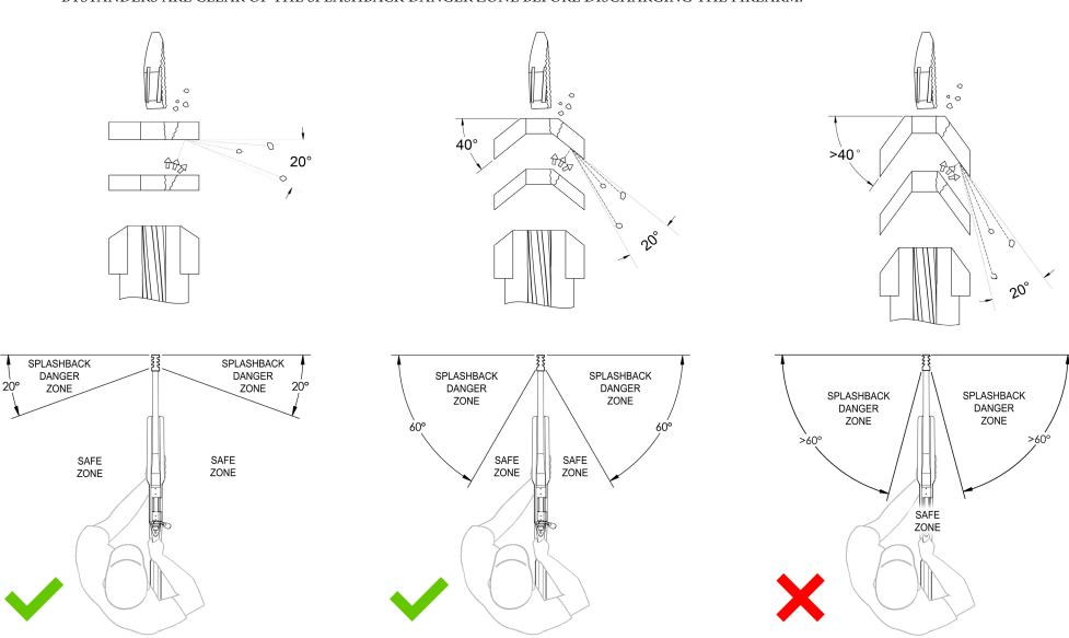
Figure 1a. Flat baffles feature a zero-degree impingement angle providing the largest safe zone.
