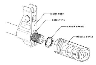
**IMPORTANT:** THIS MUZZLE DEVICE IS DESIGNED ONLY TO BE USED ON THE AK-47 RIFLE CHAMBERED IN 7.62MM CALIBER OR SMALLER.
