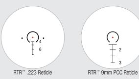
New to the TAC-R series is the RTR<sup>™</sup> (Rapid Target Reticle) for the 1.5x16S and 2x20 ACOG® models. The RTR™ .223 reticle includes a bright fiber optic/tritium 2.0 MOA illuminated center dot, BDC holds to 700 yards for .223 REM 55gr. FMJ ammunition and a 16 in. barrel length, 7.5 MPH crosswind holds at 250 yards, and 19 in. width stadia lines for ranging.
