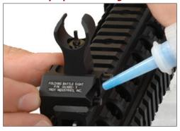
2. Apply one drop of thread locking compound to expse threads. Replace clamp and tighten screw while pushing sight forward against cross-slot.
