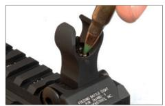
Adjustments: To move bullet impact up, turn adjustment wheel to the right/clockwise.
