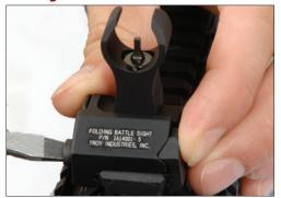
1. Unscrew clamp assembly and place sight so as to allow clamp screw to rest in foremost rail crossslot on handquard.
