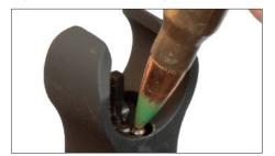
Adjustments: To move bullet impact down, turn adjustment wheel to the left/counter clockwise.
