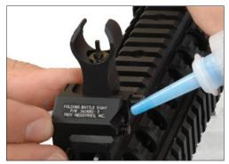
2. Apply one drop of thread locking compound to expse threads. Replace clamp and tighten screw while pushing sight forward against cross-slot.
