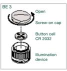
Usable replacement batteries: Button cell, 3 V, Type CR 2032
